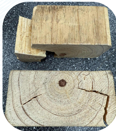
Wood fractures before glue failure; various wood types tested
