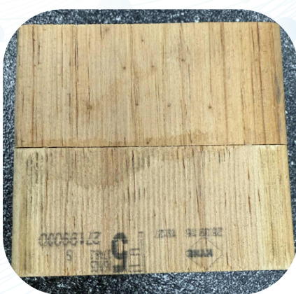
Wood fractures before glue failure; various wood types tested
